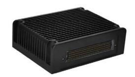
Small, smaller and even smaller, Trident welcomes their latest rugged COTS nano-small form factor (nSFF) computer, the Kestrel, into their SFF product family. The Kestrel retains the same level of environmental ruggedization and compliance to MIL-STD-810 and DO-160 specifications, including extended temperature, shock and vibration. At 60,000 feet or on the ground, the Kestrel is an ideal choice for avionic, vetronic and other military and rugged industrial applications.
