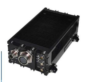
The Willet-N is a rugged ultra-SFF GPGPU AI SWaP Optimized Super computer, specially tailored for the avionic, military and rugged industrial market. It incorporates the powerful NVIDIA® Jetson AGX Xavier-based AI SOM that provides 512 CUDA cores and 64 Tensor cores, reaching 32 TOPS (INT8) and 11 TFLOPS (FP16) at a remarkable level of energy efficiency.
