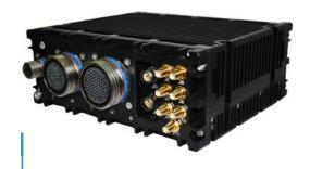
The Lanius-3 is a rugged mini-small form factor (SFF) conduction cooled computer system, specifically tailored for the avionic, military and rugged industrial market. The system offers the best utilization of size, weight and power (SWaP) in the industry and strictly adheres to commercial Off the Shelf (COTS) standards in the industry. Though its small in size, its feature rich & best in class embedded computer.
