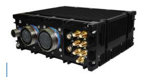
The Lanius-5G is a rugged micro-small form factor (SFF) conduction cooled computer system, specifically tailored for the avionic, military and rugged industrial market with 5G & WiFi-6e modules preconfigured. The system offers the best utilization of size, weight and power (SWaP) in the industry and strictly adheres to commercial Off the Shelf (COTS) standards in the industry. Though its small in size, its feature rich & best in class embedded computer.
